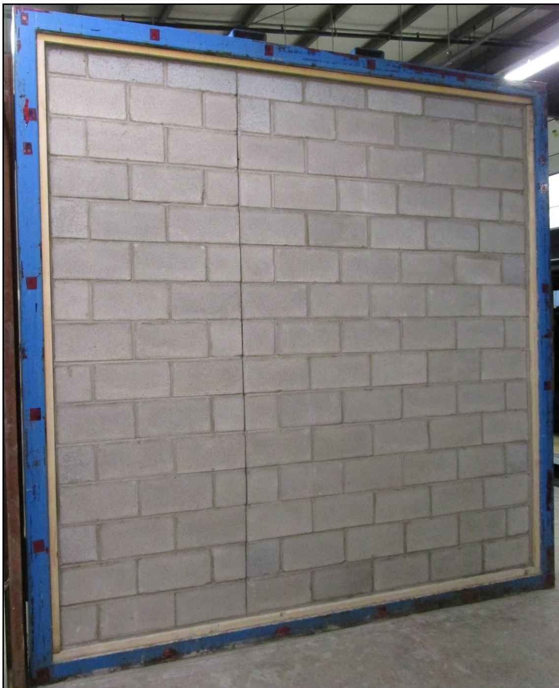
Photo J1 – Opaque CMU wall section prior to product application
