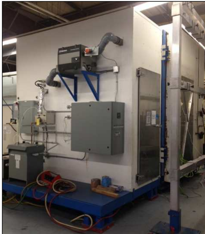
Figure 2 – General Specimen Installation between Warm Side and Hygrothermal Chamber
