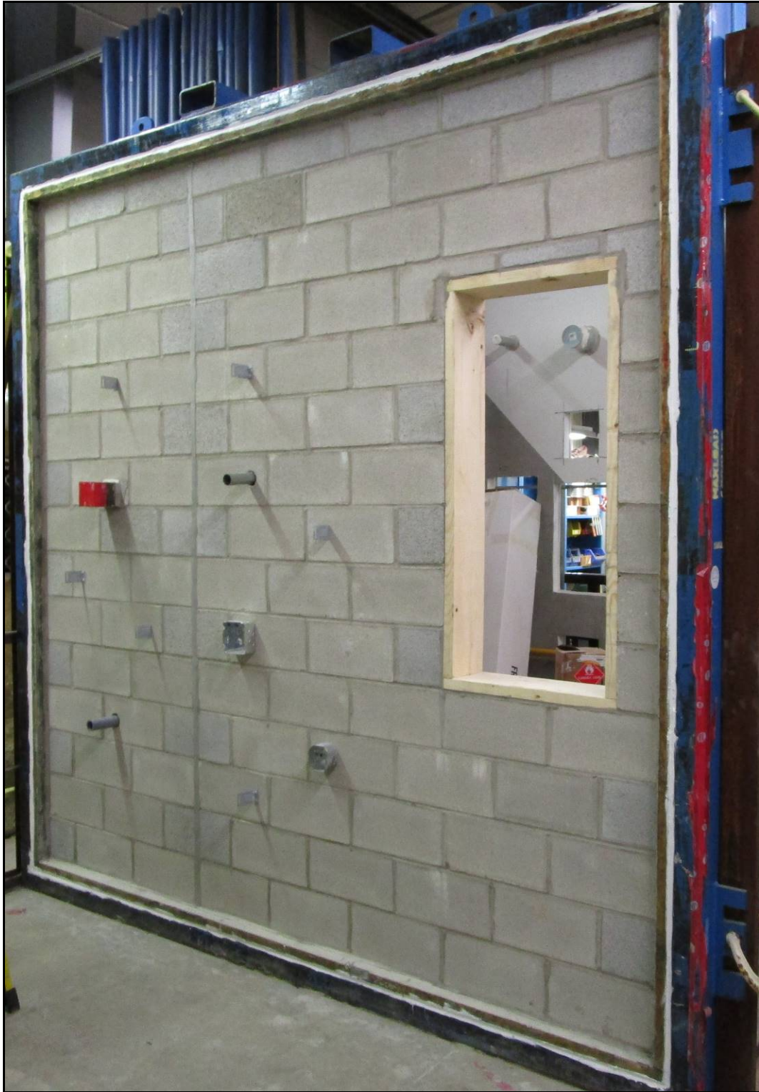
Photo K1 – Opaque CMU wall section prior to product application
